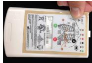
4. Take Header and internals assembly and slide them into the new case. Connect the ribbon cable and reinstall the set screw. Use original screws and new screw covers to reattach header to unit
